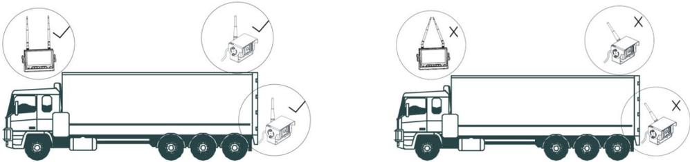
2) Magnet based extension antenna should be attached on the top of the vehicle. Make sure there is no obstacle around or between 2 antennas.
