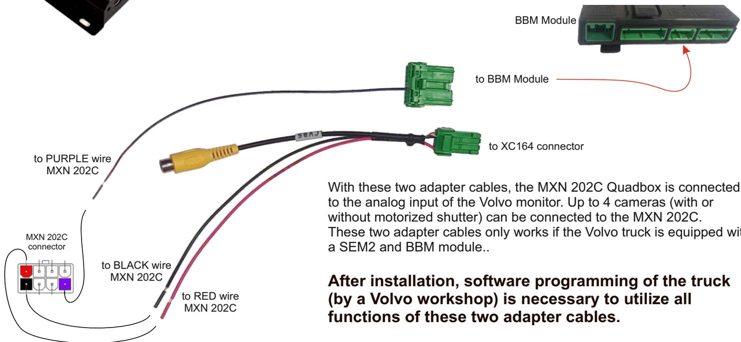
With these two adapter cables, the MXN 202C Quadbox is connected to the analog input of the Volvo monitor. Up to 4 cameras (with or without motorized shutter) can be connected to the MXN 202C. These two adapter cables only works if the Volvo truck is equipped with a SEM2 and BBM module..
